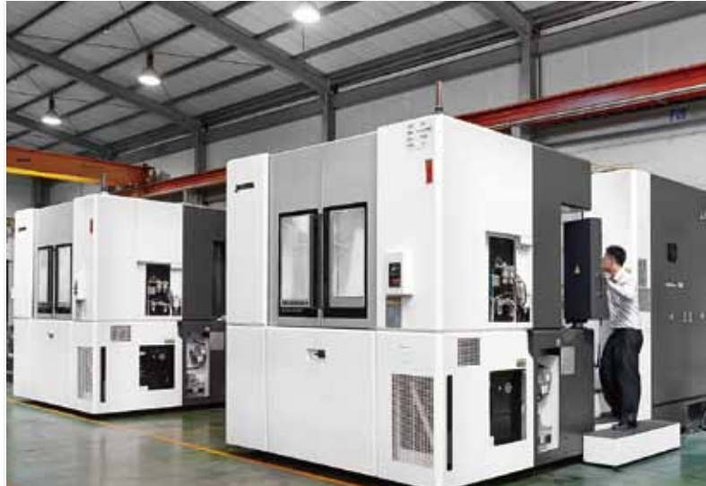
Adopting CNC Horizontal Machining Center for Housing and Tool-Disc Machining.
