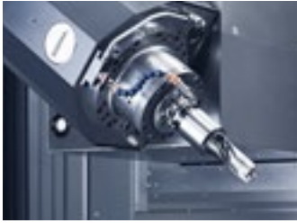
Air blowing function to the tool on main spindle nose.
