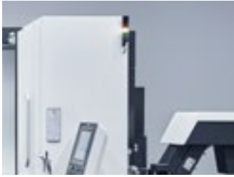
3 light tower acoustic signal.
