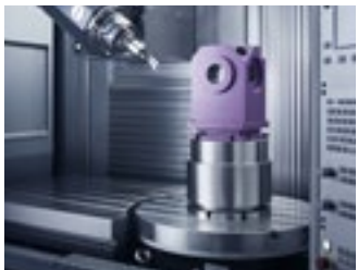
ø800 mm integrated rotary table (STAR 1500).
