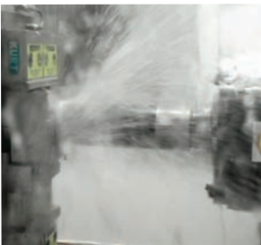
Up to 1000psi Coolant Thru the Spindle Available
