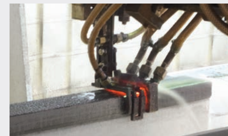
Induction hardened solid box guideways with linear scale feedback on all axes with twin ballscrew design in X, Y & Z axes.
