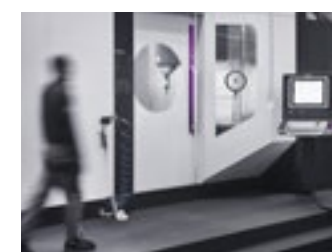
Totally encapsulated working area and safety windows.
